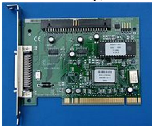
A typical 32-bit, 5V-only PCI card, in this case a SCSI adapter from Adaptec
